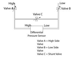
For differential pressure measurements at high line pressure (350 psig max.), it is recommended that the pressure sensor be installed with a valve in each line, plus a shunt valve across the high and low reference pressure ports as shown.
